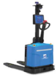
3D SLAM Lightweighted Pallet Truck (LXST15-D)
