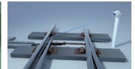
Railway Turnout Deformation Detection Solution
